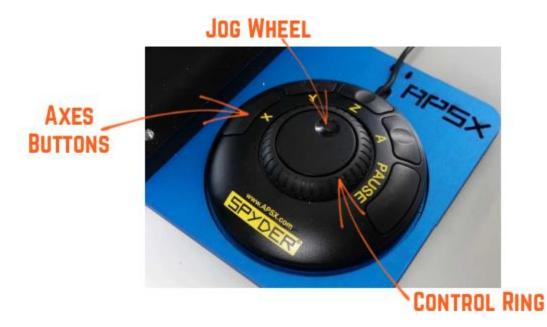
The pendant allows precise control of the machine's travel speed. For example, manually touching off the end mill to your workpiece and zeroing the X, Y and Z-axis requires small adjustments at low speed. It increases efficiency on the jobs that require a difficult setting of the workpiece and the tool.
