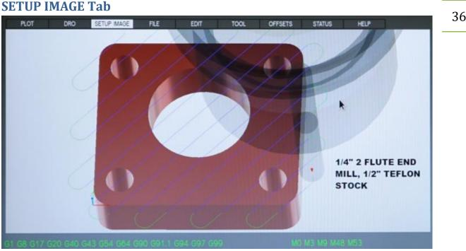
If you create and save a picture with the same file name as the g-code program, it will show it on this tab. The picture file name should have png extension (lower case) at the end. You can show the setup layout and add some critical notes to it. The idea is to make the setup process easier for you by using this cheat sheet.
