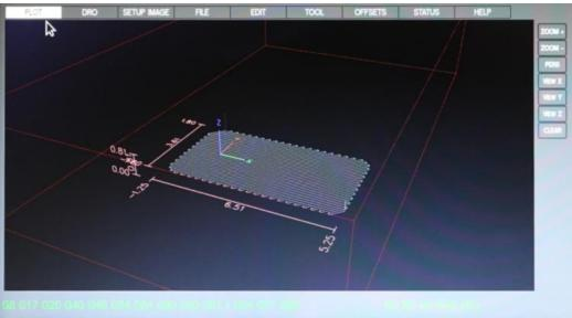
The PLOT tab displays a graphic representation of the work coordinates and the toolpath in the g-code loaded. The preview lines are in white, and the toolpath as it is milled is red in color. There are preview buttons on the side: ZOOM, PERSPECTIVE, VIEW X-Y-Z, and CLEAR.
